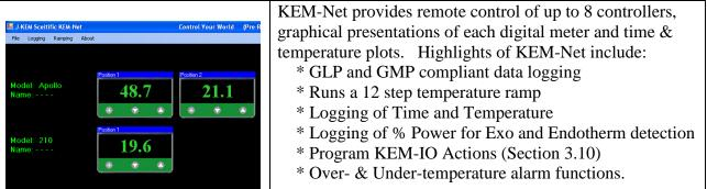
KEM-Net also includes a virtual comm port driver that provides a simple ASCII interface to operate and data log the controller from LabView or other software packages.
